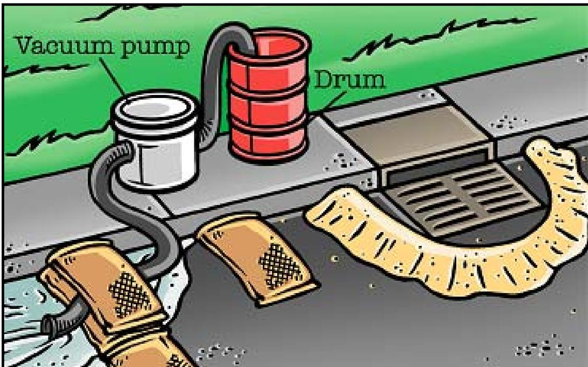
2. *A vacuum system can be set up to constantly suction up contaminated liquid as it reaches the containment dam.*
